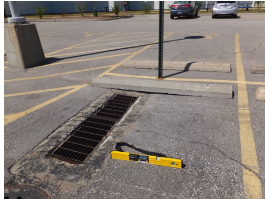
Figure 4. SLSC Accessible Parking with 8.1% Slope
